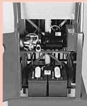
The Maxi-Lift's® smooth electro/hydraulic system is powered by 2 batteries.
