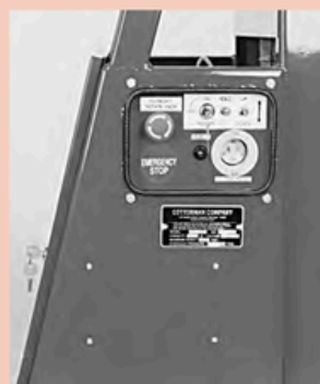
Control center in base includes a master key lock. An emergency stop button. Platform motion controls and 120 VAC input for platform outlet.
